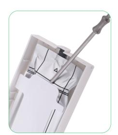
Fast metering of residual oxygen content in closed containers
